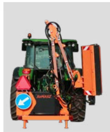
Unit in transport position - rear bumper with noticeable road lights.
