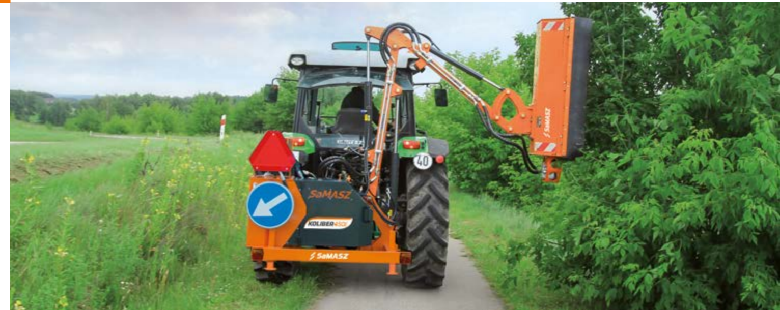
Work reach of KOLIBER 400 extension arm with LAMA 120 [cm] mowing head
