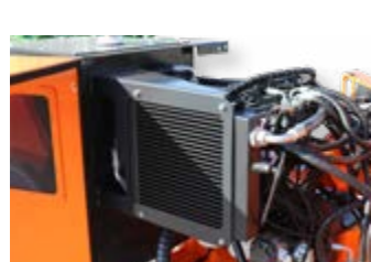
Within the hydraulic system, an oil radiator is installed which protects the unit from overheating.
