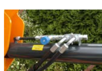
Additional stop valve protects the arm from falling even if hydraulic hose gets damaged.
